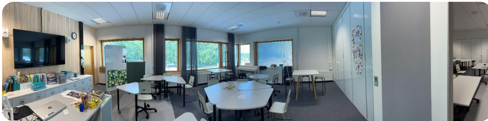
Figure 43. Walls that can be opened and closed between classrooms to enable co-teaching- Kortepohja daycare-school ©Markku Lang
